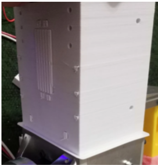
Brim and support material used on 3D printed part
