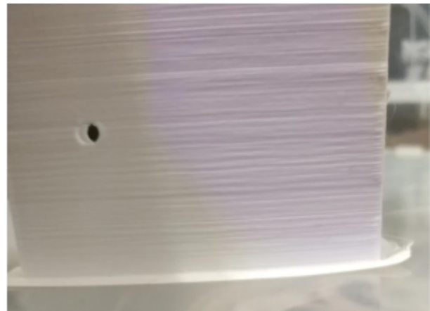
Evidence of warping on 3D printed part
